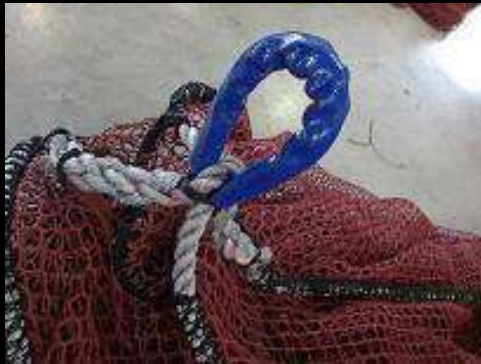
Rope looped + pipe protection
